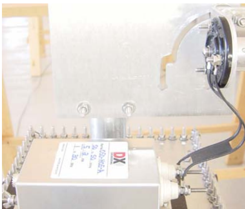
Figure 2 Insulated Balun System for Use with Hustler Antenna without Radials. Even though this is not recommended, we realize that many people do it anyway, so this is a way to reduce the resulting current on the feedline.
