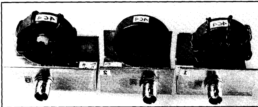
Fig 3-9—Transformers used in the comparison of the performance of twisted pair windings v tightly wound and twin-lead windings.
